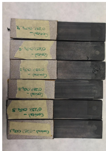
FIGURE 10 Metal-elastomer coupons to perform Peel-off tests
